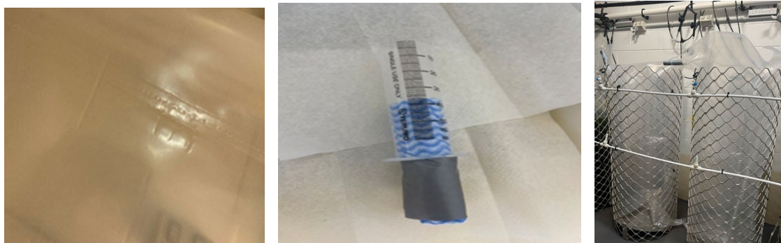
Figure 5 – Left – visually inspect the bag seams for any deformities or weaknesses, Centre – a modified syringe with sterilisable cloth cap, Right – the syringe/cloth cap taped into the corner of a bag.
