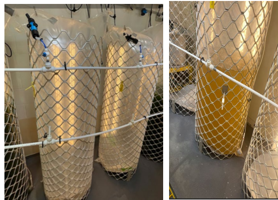
Figure 7 – Left – example of the mini-filter and John Guest seawater tap feeding filtered seawater into a bag, Right – aeration (bottom right) and sampling ports created with pipette tips and duct tape.
