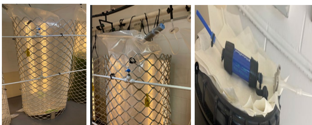
Figure 6 – Left – 400 L bag with the bottom corners protruding from the cage, Centre – filtered air being delivered to inflate the bag, Right – mini filter set-up through which filtered seawater will be delivered to the bag.
