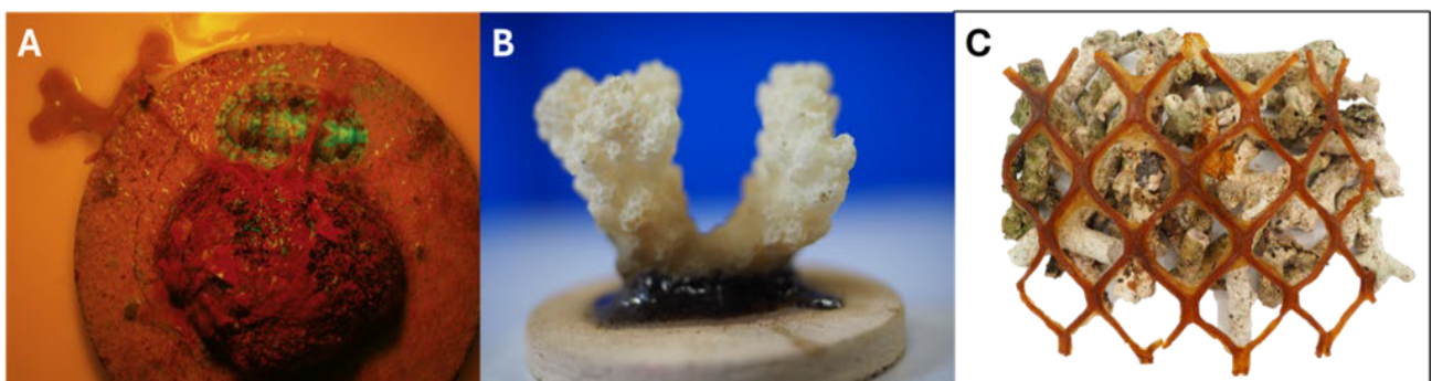
Figure 5: Bioadhesive tests and applications. A) 90-day ecological and microtoxicity trial at the Australian Institute of Marine Science (AIMS) National Sea Simulator (SeaSim). Five cm diameter ceramic tile with bioadhesive is fouled with fibrous and fleshy algae, and crustose coralline algae; a chiton is adjacent at top. Image taken in UV light. B) Example of bioadhesive used for coral fragment attachment test. C) Plan view of bioadhesive moulded mesh for direct substrate stabilisation.
