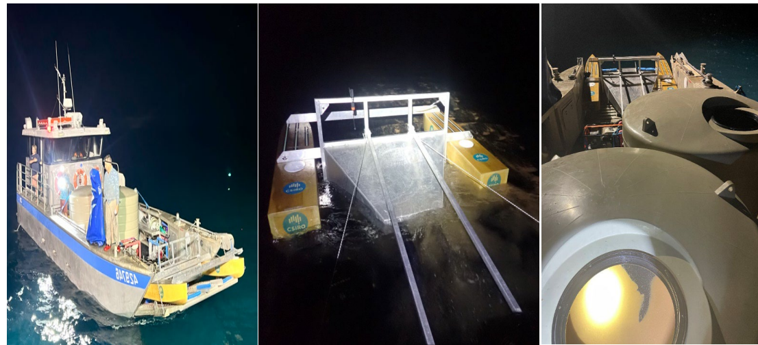
Figure 6: Collections of wild coral spawn slicks directly from the water surface to two 1,500 L tanks onboard a barge using diaphragm pumps and a floating intake mouth. Far right image shows direct transfer into a larval pool for culturing.
