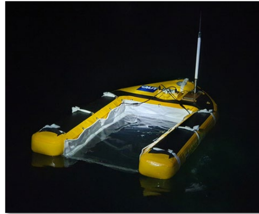
Figure 5: An ASV fitted with the spawn catching net during operation (Mou et al. 2022).
