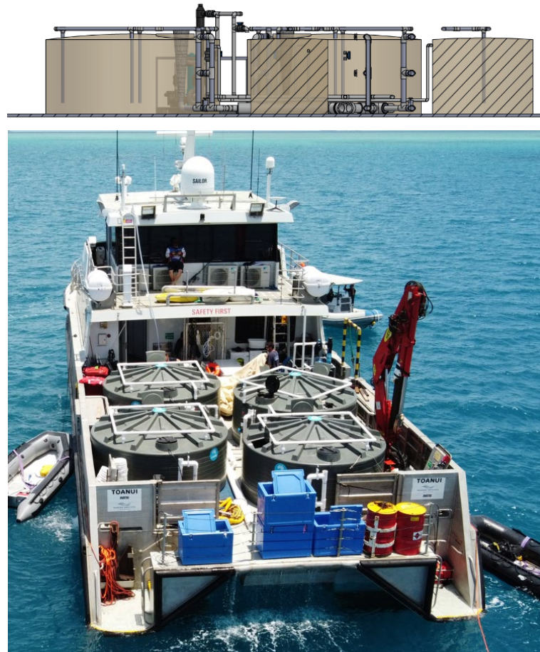
Figure 17: Computer-aided design drawing and image of the flow-through vessel-based aquaculture system. Each tank holds 10,000 L of seawater.
