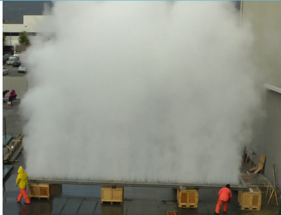
Figure 22: Spray test of ~400 nozzles from a MeeFog™ nozzle manifold with 1600 nozzles.
