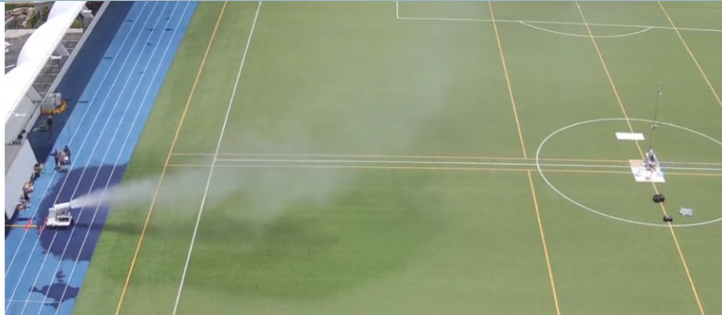
Figure 21: Fog plume moving toward instrument stand with some shading visible under plume.
