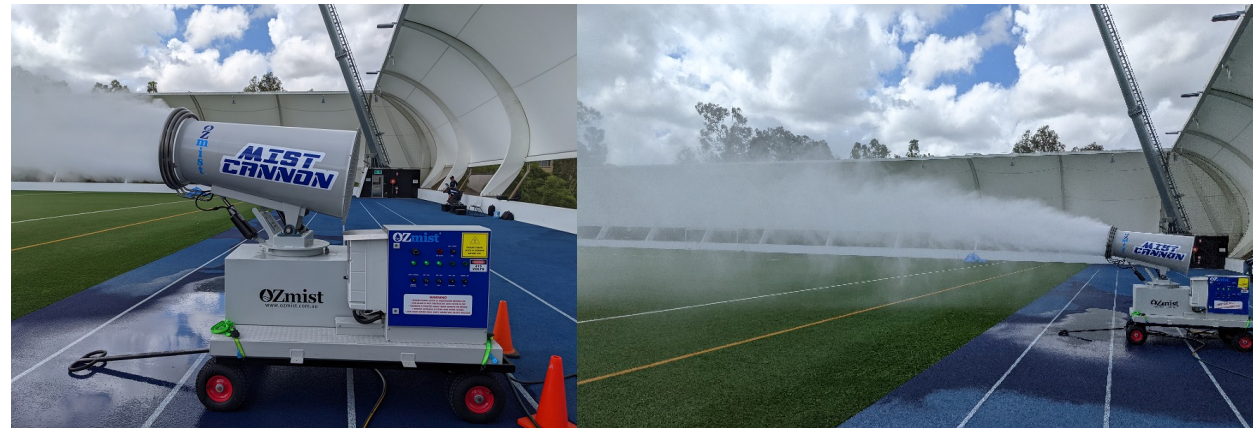
Figure 19: Initial POC Fog Cannon (Fogger V1) - left view showing control pane (Left). POC Fog Cannon Spray during the land trials at the Queensland University of Technology (QUT) soccer stadium, Brisbane (Right).
