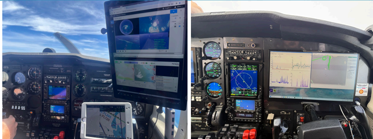
Figure 3: The flight mission scientists aircraft panel pre and post avionics upgrade. Left) Steam gauges and ad-hoc science displays using tablets in the cockpit. Right) The upgraded panel with modern avionics and panel mounted navigation and science displays.
