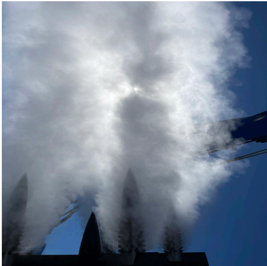
Figure 1: Marine cloud brightening sprayer during operation.
