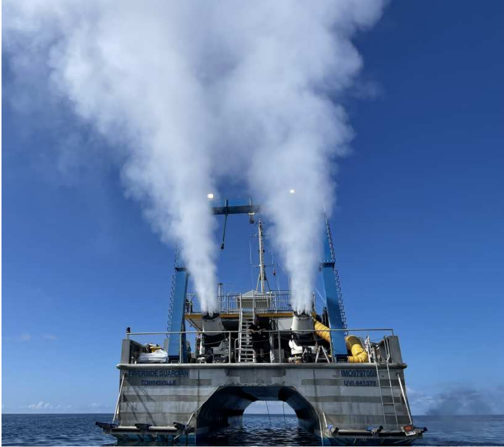
Figure 1: Marine cloud brightening sprayers in operation on the Great Barrier Reef, 2025.
