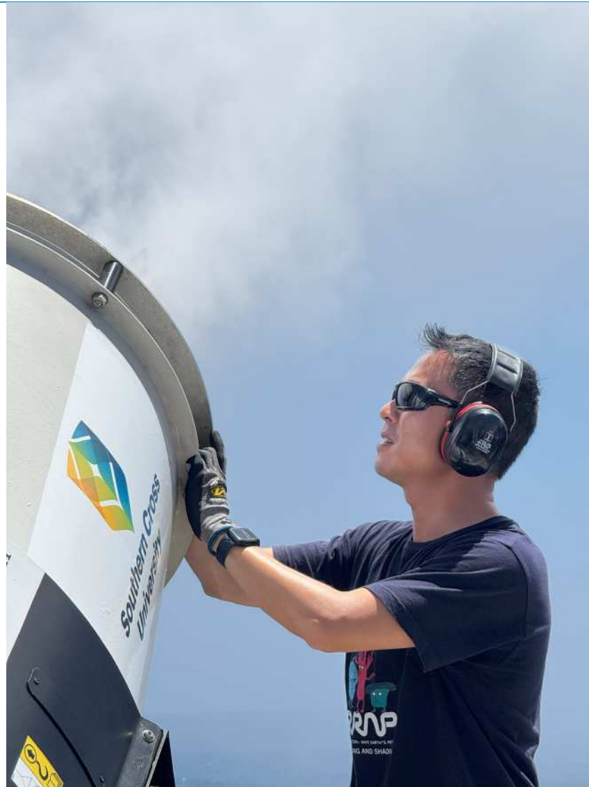
Figure 3: Cheng Chen checking the nozzle tower of the marine cloud brightening sprayer during field tests in 2023 on the Great Barrier Reef.
