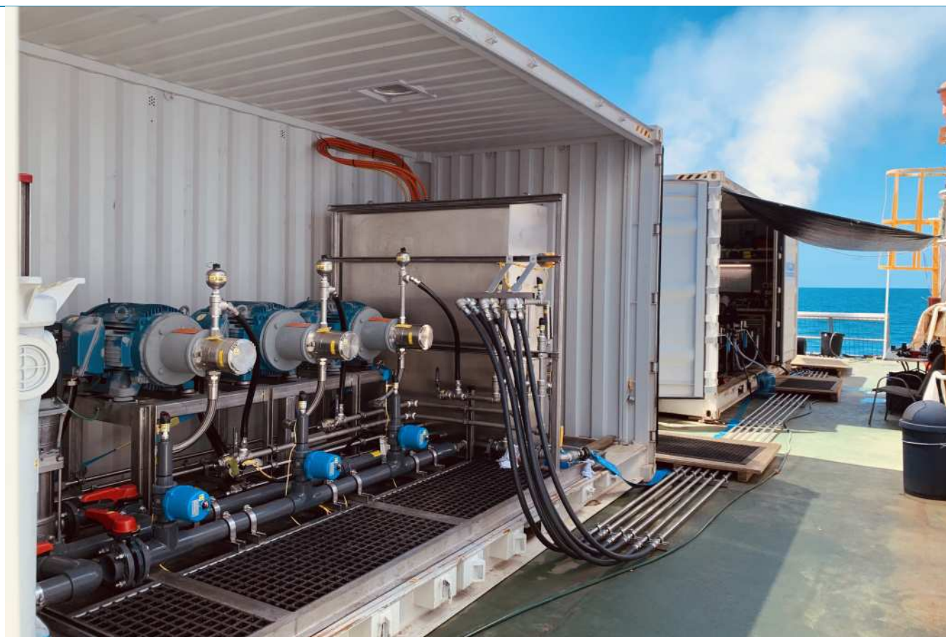
Figure 7: Marine fogging infrastructure set up on a research vessel during field trials in the Great Barrier Reef, 2023.
