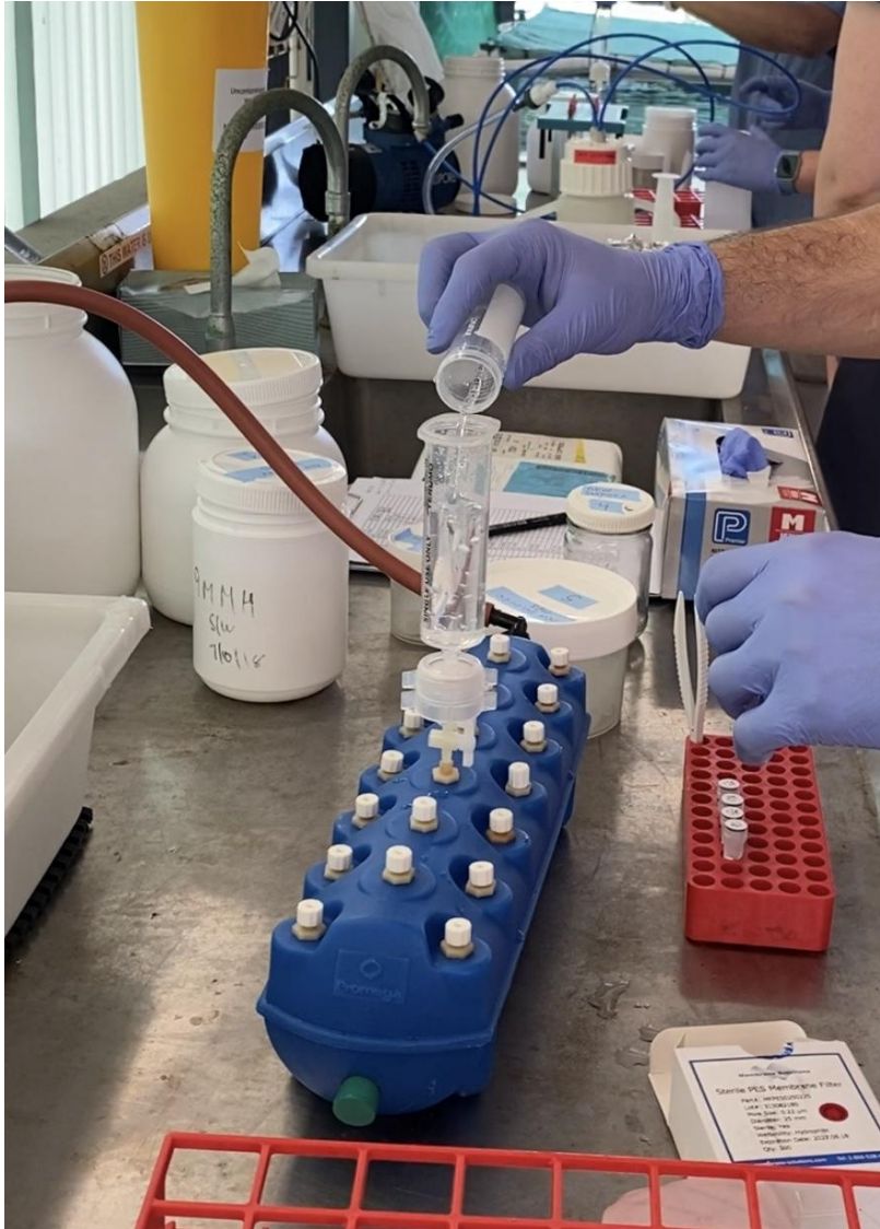
Figure 2: Overview of the filtration station for sampling of seawater-borne bacteria using a filter membrane and vacuum pump.
