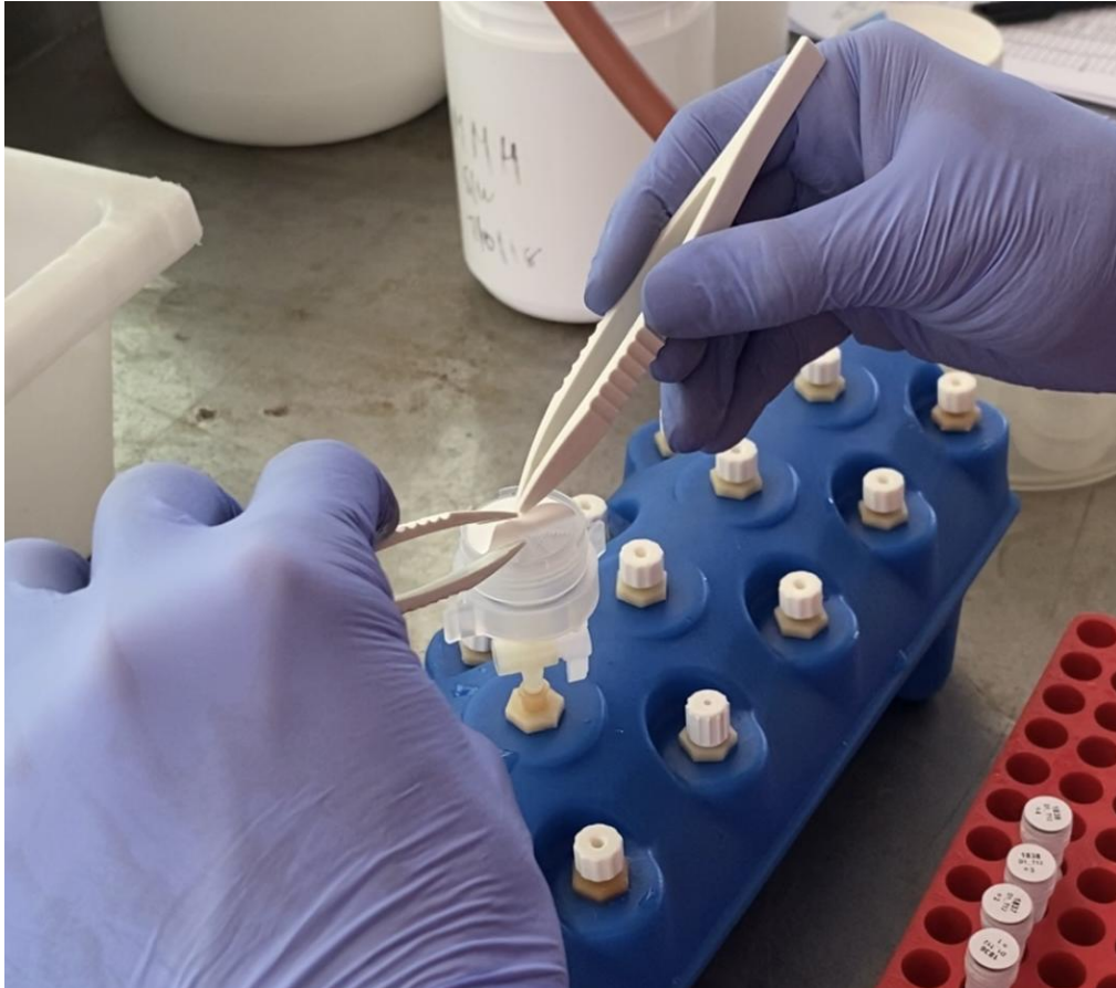
Figure 3: Removal of the filter membrane for microbial sampling from the filtration unit.
