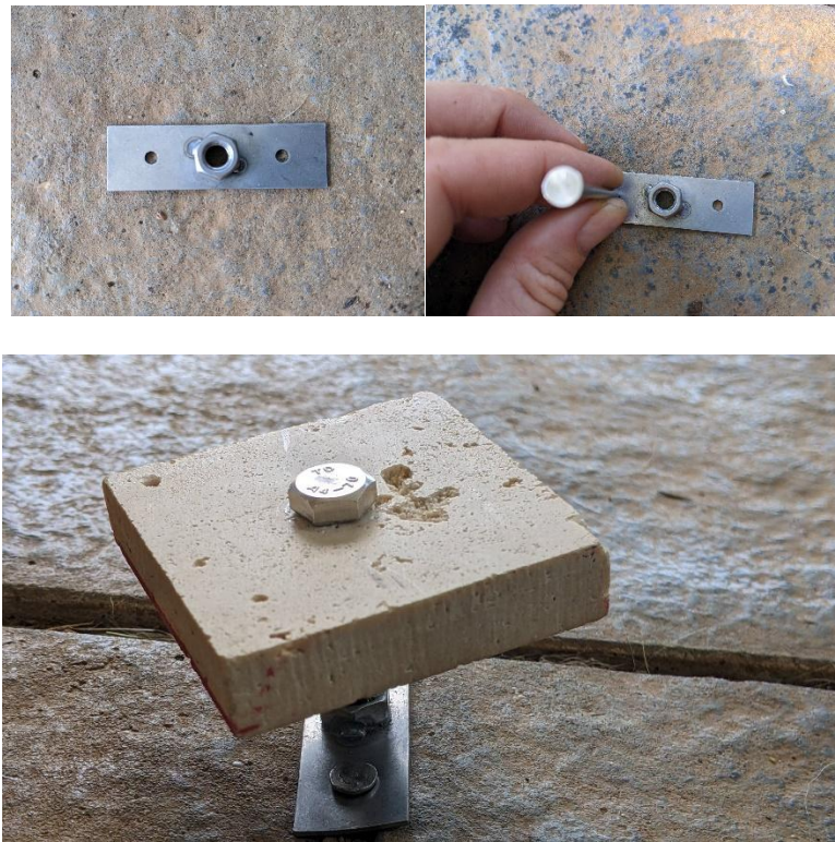
Figure 8.1.3: Settlement tile 'mini' baseplate deployment
