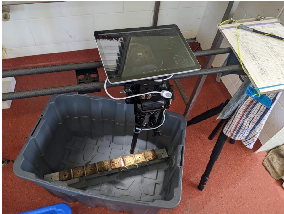
Figure 8.1.9: Photography set up to take high resolution photographs of tiles
