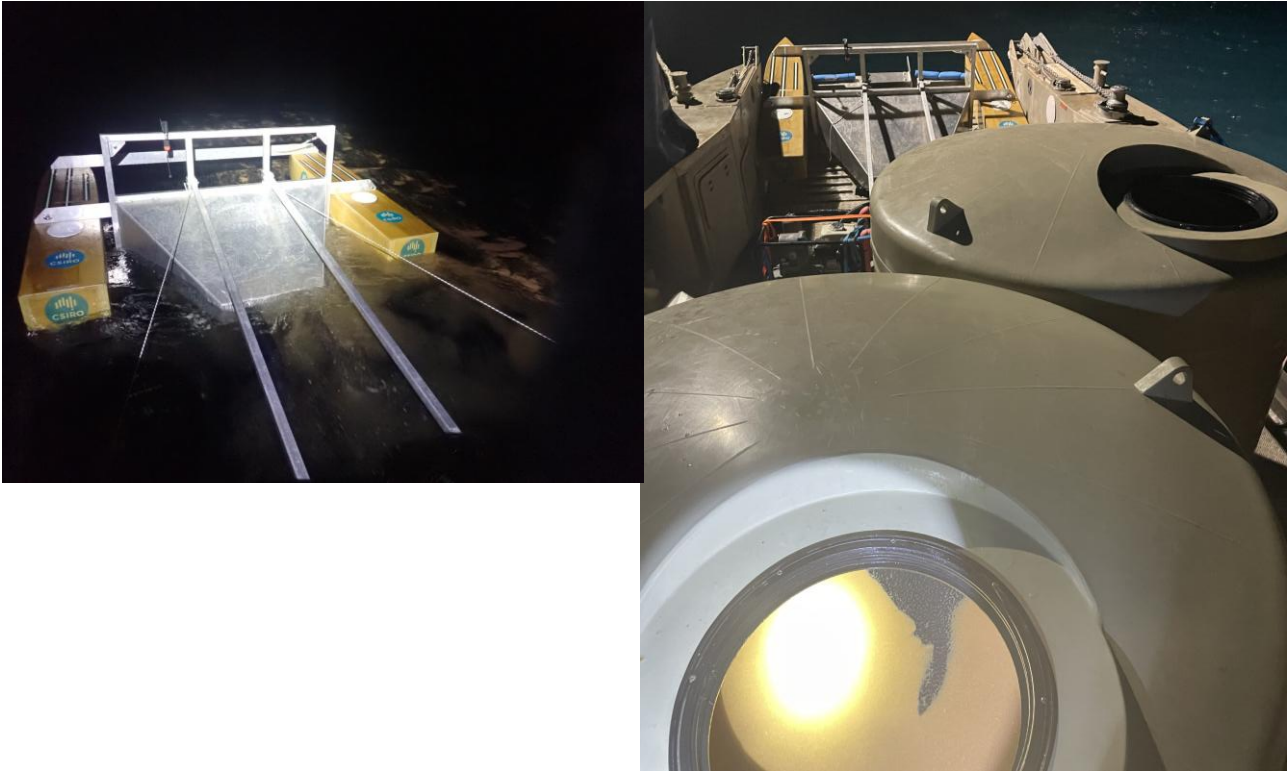
Figure 5.2.2: Spawn sucker with updated floating collection mouth during collection, and rainwater tanks full of spawn following collection during field collections at Eyrie Reef in 2023 (Photos: G. Carlin, C. Doropoulos)
