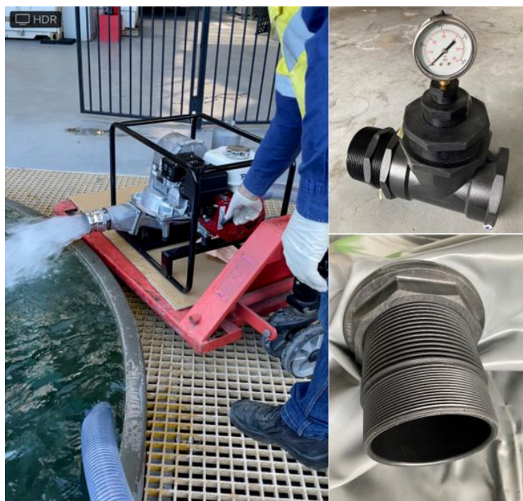
Figure 5.2.5: Setup for camlock fittings and pressure gauge on pumps
