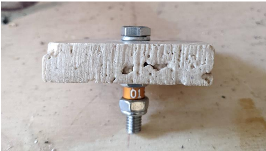
Figure 8.1.2: Settlement tile assembled on bolt with tag
