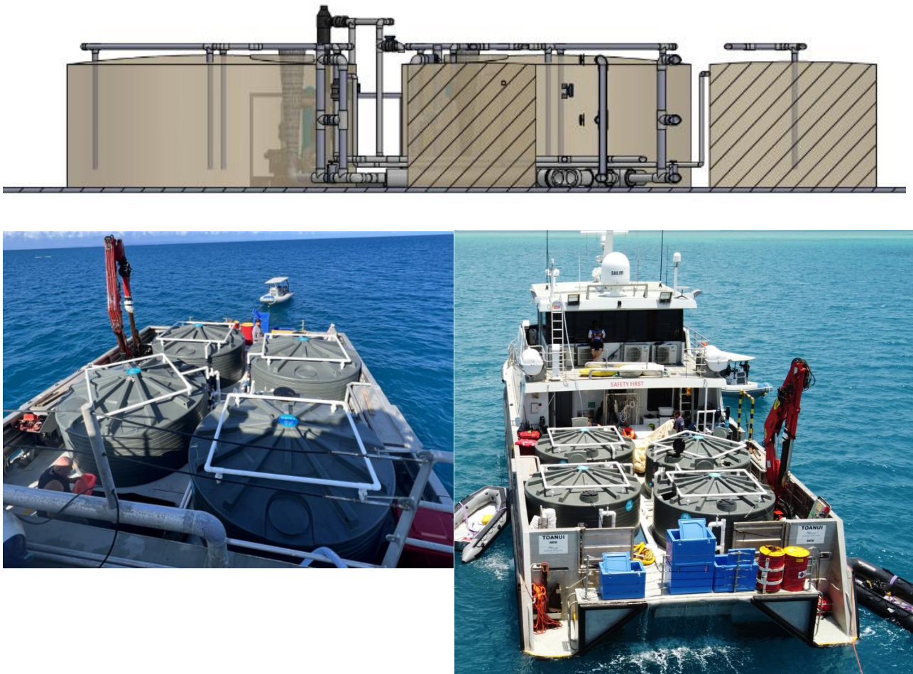
Figure 6.2.1: CAD design drawing and images of the flow-through vessel-based aquaculture system on the aft deck of Toanui in 2023. Each tank holds 10,000 L of seawater (Photos: C. Doropoulos, North Marine)
