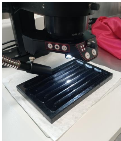
Figure 1. Bogorov counting chamber under a stereoscope to perform Artemia counts (Photo credit: Sara Godinez-Espinosa).
