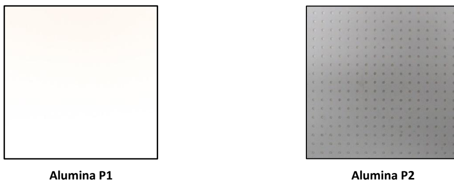
Figure 3: Partially Sintered Alumina Tiles with artificially modified surface porosity.
