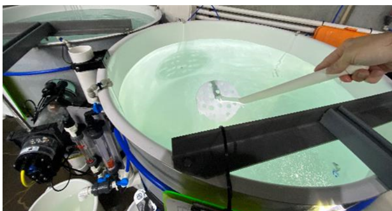
Figure 7. Homogenising the culture of a tank with removed filter using a PVC 'larval culture plunger' while harvesting to a graduated bucket. Photo credit: Dr C. Brunner.
