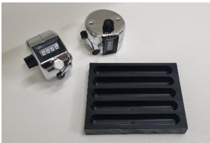
Figure 6. CAD counting tray and clickers/counters for assessment of larval culture density. Each channel can hold 3-5 mL of seawater, depending on the version. IP & photo credit: Australian Institute of Marine Science.
