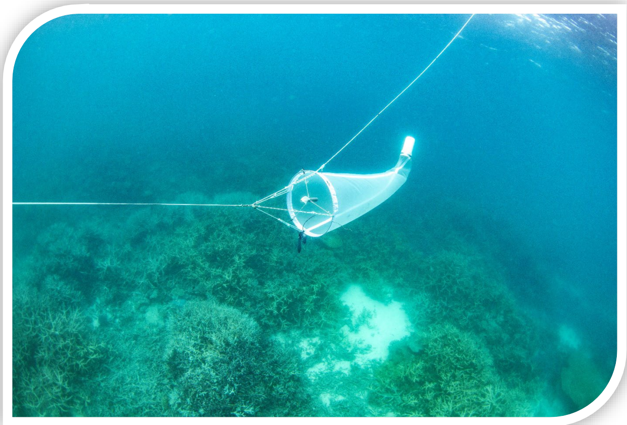
Figure 1 Deployed plankton net during tow along Heron Island reef slope. Note the flow meter in the centre of the mouth of the net, the weights at the bottom of the mouth of the net, and the rope coming from the top of the net has a buoy on the surface. The relationship between the buoy, the weights, and the tow speed influence the depth of the plankton net in the water column during a tow.
