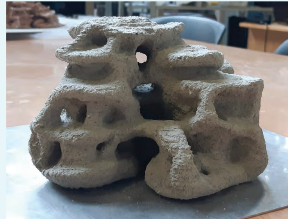
Figure 83. 3D printed reef structure made of local materials – “Reef Arabia” deployed in Bahrain. Source: David Lennon
