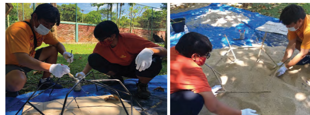
Figure 115. Coating Reef Stars with boat resin (left) followed by coarse sand (right). Source: Marthen Welly, Coral Triangle Center
