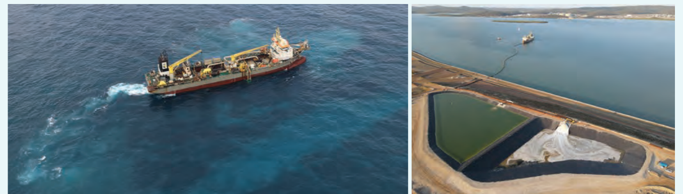
Left: Figure 42. Trailer Suction Hopper Dredge – “Gateway” Source: © Great Barrier Reef Marine Park Authority Right: Figure 43. Floating pipeline transporting dredged materials from the dredger to onshore ponds in Gladstone. Source: © Great Barrier Reef Marine Park Authority
