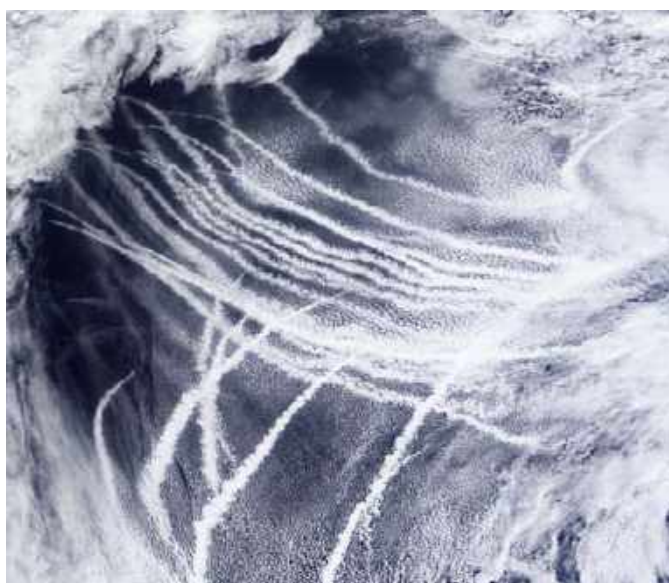
Figure 5: Cloud brightening due to marine ship exhaust is a visually detectable occurrence due to the high albedo change which occurs under certain atmospheric conditions. These conditions are not often present on the Reef, but modelling (see Report T14- Environmental Modelling of Solar Radiation Management) has indicated that low-level clouds on the Reef are amenable to a lower intensity of brightening. Image credit: NASA .
